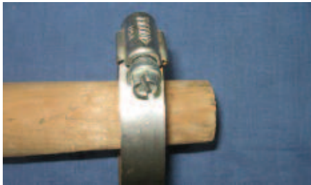
Clamp over flattened end of pole. The flat end makes it much easier to securely clamp the pole to the frame.
