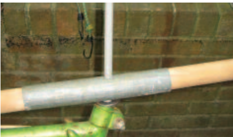
Rod passing through the reinforced part of the pole and into the seat tube. The bends in the rod allow it to jam tightly in the tube which makes controlling the bike easier.
