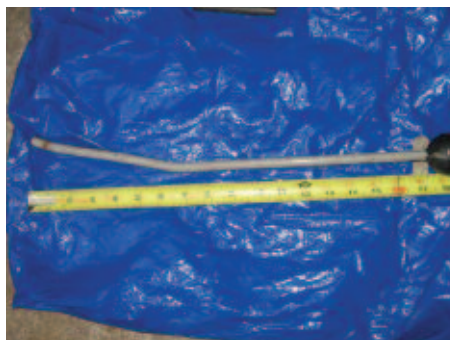
The rod should be at least 18" long with slight bends, about 1" and 7" from bottom end.
