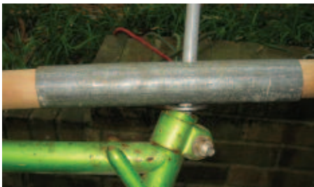
Washer between seat tube and pole is essential. Metal reinforcement on pole and washer spread out weight, reducing stress on the pole. Heaviest load should go between rod and clamp.
