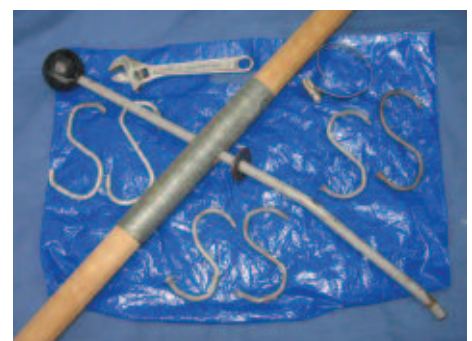
The rod passes through the pole and the metal tube reinforces the pole.
