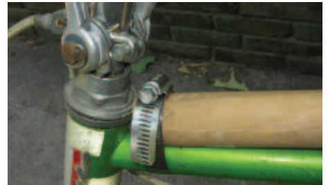
The pole is tightly clamped to the frame. Any wiggle here can cause the pole to break or the load to come loose.
