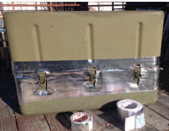
Sealing Outside of Aluminum Clamshell Box for EMP protection
