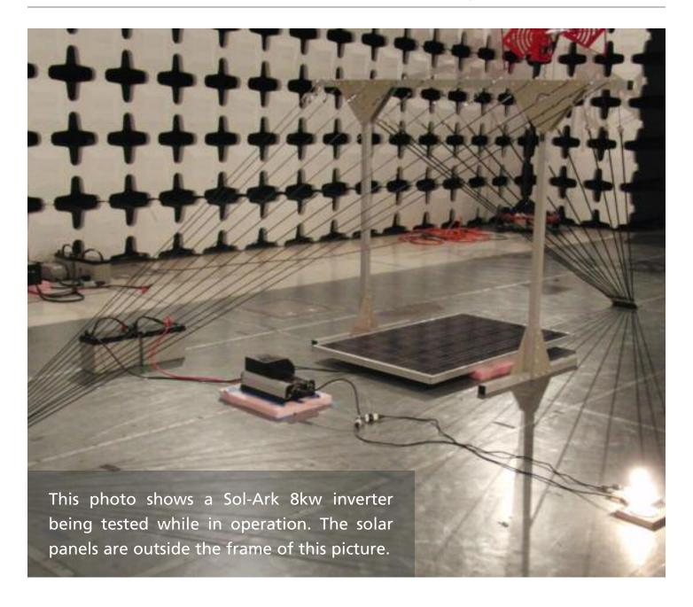
nent-they don't do so well with directly-induced surges through the wiring), the peace of mind of having panels that can soak up hit after hit after hit of EMP on powsimulators dishing up erful 100,000 volts per square meter cannot be measured. Sol-Ark owns their own simulators, but have submitted their complete solar generation systems to independent laboratories for testing. Shielding panel wiring inside steel conduit may increase the survivability of a solar array.
