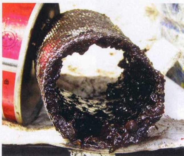
As fuel deteriorates in storage, the residue from degradation begins to plug fuel filters. The photo of the filter above was taken from a diesel powered pumping station designed to ward off flooding in a low lying area. With a failure in the system, hundreds of homes are put at risk.
